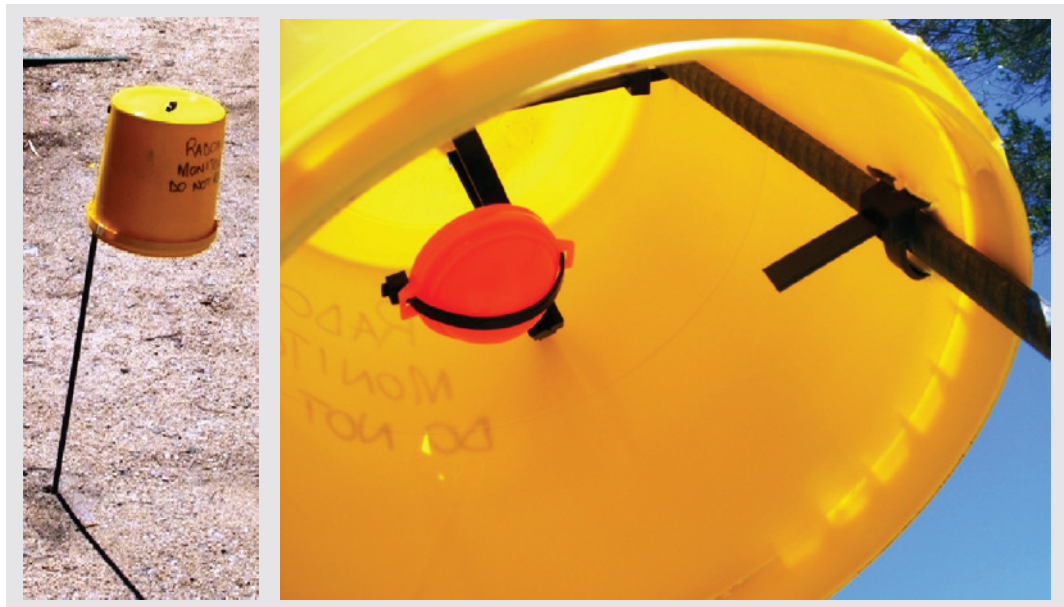
Figure 2: Photograph showing how a radon cup is affixed to the inside of the plastic bucket 1 m above ground.
